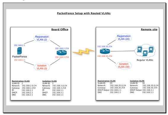
For dhcpd, make sure that the clients DHCP requests are correctly forwarded (IP Helpers in the remote routers) to the PacketFence server. Then make sure you followed the instructions in the <u>DHCP and DNS Server Configuration (networks.conf)</u> for your locally accessible network.
